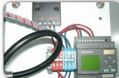
Gel battery, logic controller (above) and air solenoid valve (below).
