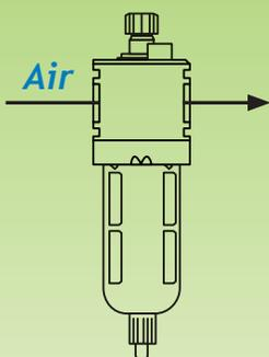
Pressurized air enters the unit and passes through an inlet valve to the oil-filled polycarbonate bowl at the bottom. The air is infused with microscopic droplets of oil, then exits the unit through a hole connected to the 3" long nipple and enters the cylinder through the intake. Reciprocating action of the cylinder's drive rod regulates opening and closing of the entry valve.
