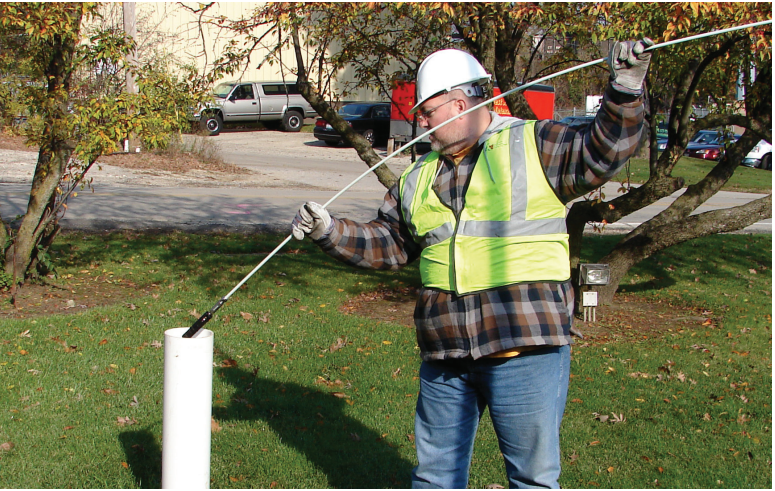
Using piston and rod to determine well depth
