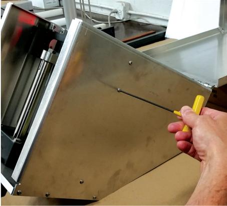
Remove cover screws with Allen wrench
