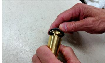
3) Work blade around piston to remove.
