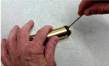
1) Insert flat blade of small screwdriver under seal.
