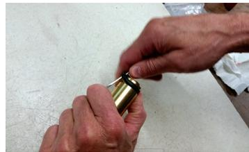
7) Insert screwdriver through seal.
