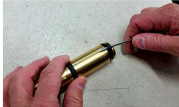
2) Push blade underneath and through seal to bring up from groove.
