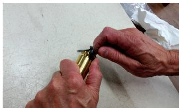
6) Press new seal into groove.
