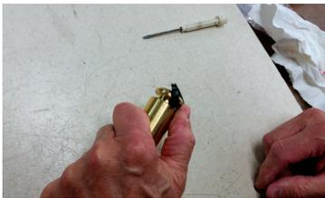
5) Clean piston before inserting.
