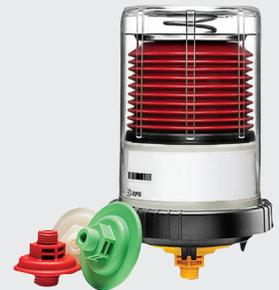
The screw-in cartridge is made from recycled polymer and can be replaced in 60 seconds. Users choose from four time-release settings, up to 12 months. The auto lube operates to 140 psi.
