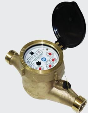
Velocity-type single-jet model with copper-alloy housing. Maximum operating pressure 150 psi. Sizes: ¼ in. to 2 in.
