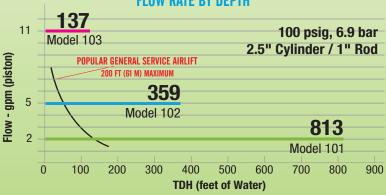
Blackhawk positive-displacement piston pumps provide uniform flow, unaffected by depths. General service airlift performance diminishes significantly as depth increases.
