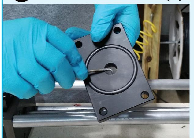
Using pick tool, remove seals from cartridge and discard. Inspect cartridge for wear. Place reusable parts in drum with paint thinner for cleaning soak.
