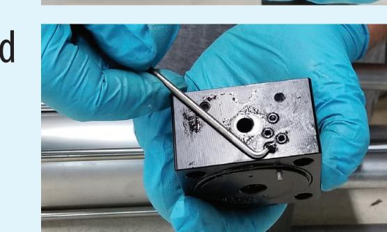
Remove cylinder, drive rod and cylinder head
