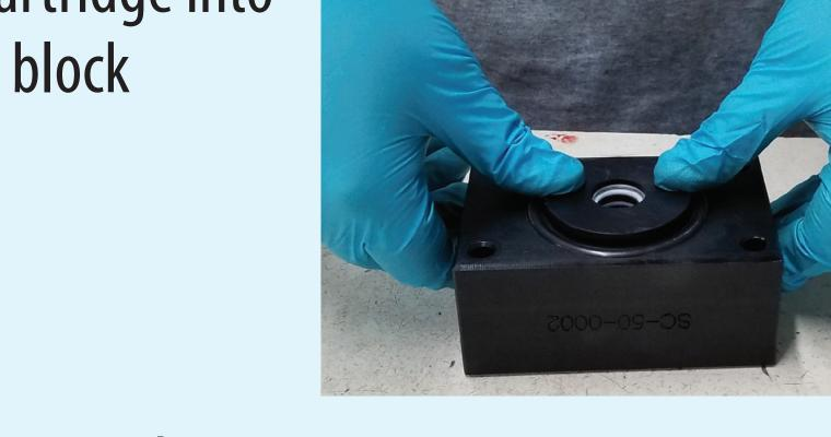
Insert new seal into auxiliary seal plate
