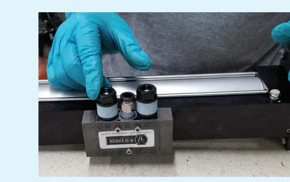
Attach seal plate, stuffing box block and mounting plate
