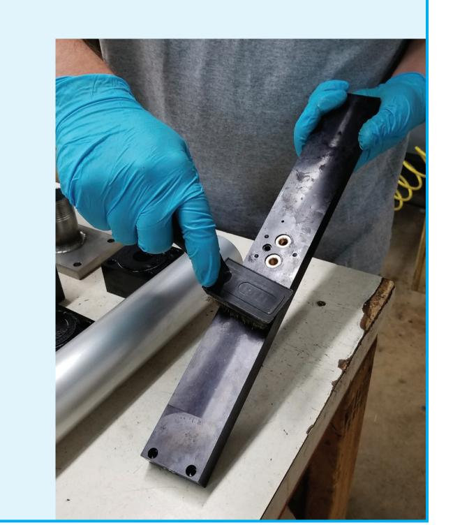
When parts are clean, the driver is ready to reassemble.
