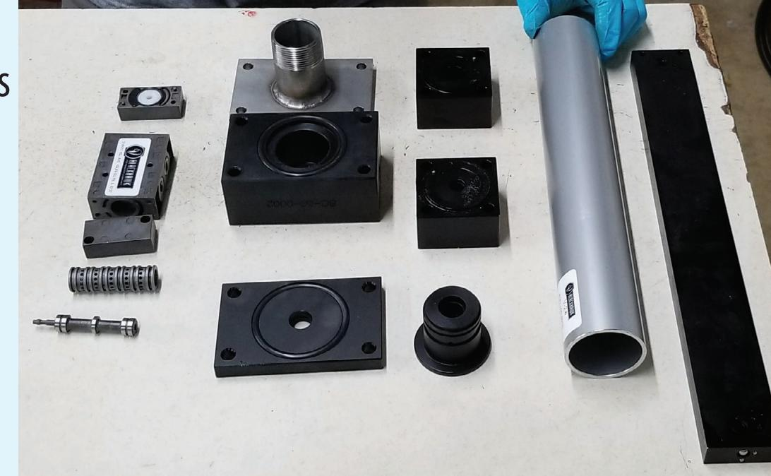
After soaking, further clean parts with wire scraper, CLR & penetrating oil as needed
