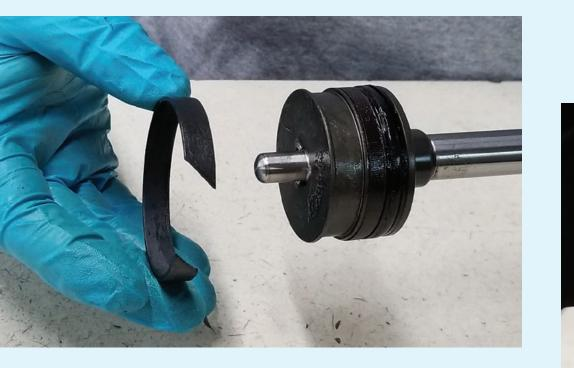
15 Using synthetic grease (small tube), lubricate both ends inside cylinder
