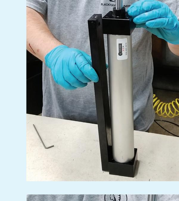
screw cap onto manifold
