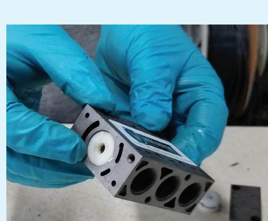
Using #3 metric hex, attach valve end caps on
