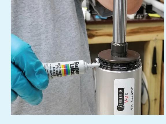
Insert piston and rod fully into cylinder with force if necessary, using rubber floor mat; do not strike on bare concrete
